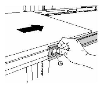
Figure 41: Sliding the Chassis towards the rear of the Rack
